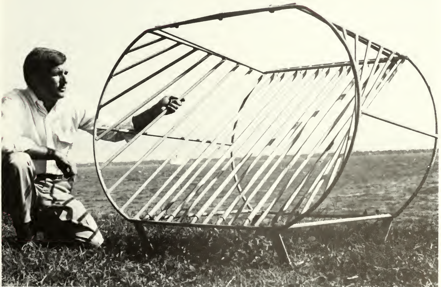
A "TED" FOR SHRIMPERS — Jack Keener, a specialist with the Sea Grant Marine Extension Program of Clemson University, shows a TED, a device that can keep turtles from drowning in shrimpers' nets, increase shrimp catch and save fuel. (CU Newsphoto)
